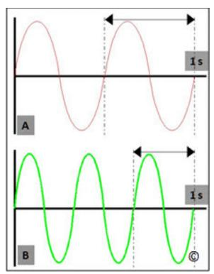
**Figure 1.1**: Frequency of sound is the number of cycles per second (s) and is expressed in Hertz (1 cycle / sec). In Wave A, the frequency is 2 cycles per sec or 2 Hertz and in wave B the frequency is 3 cycles per sec or 3 Hertz. The double arrows denote sound wavelengths, described in figure 1.3.
