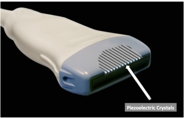
**Figure 1.4**: Piezoelectric crystals shown within a transducer. Note the symmetrical arrangement of the crystals. This figure is a diagrammatic representation, as the crystals are typically much smaller than shown. Figure 1.4 is modified with permission from the Society of Ultrasound in Medical Education (SUSME.org).
