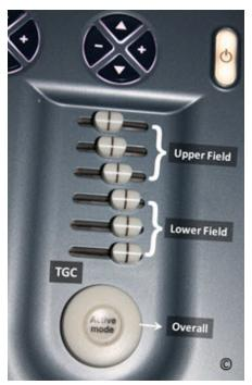
**Figure 2.12**: Time Gain Compensation (TGC) on an ultrasound consol. The upper and lower knobs adjust brightness in the upper and lower fields respectively (labeled). The overall knob (labeled) adjusts brightness in the whole image.
