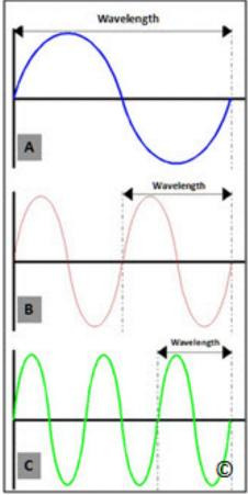
Figure 1.3: The wavelength of a sound wave is the length of a wave and is defined as the distance of a complete cycle. It is designated by the symbol lambda ( $\lambda$ ), and is expressed in mm. In this schematic, 3 sound waveforms are shown with respectively shorter wavelengths from A to C.
